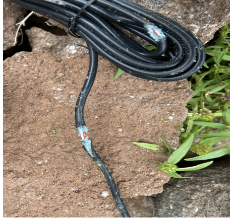
Fig. 8: Chemical weathering of temperature sensor
