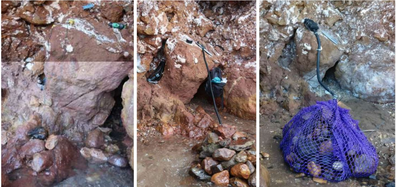
Fig. 3 Temperature measurements of the hot spring opposite Green Island, in January 2018 (left), November 2018 (middle) and February 2019 (right). Temperature probes are buried in the ocean bed and covered with rocks to keep them in place. The data loggers are the small yellow cases mounted on the rock above the spring and housed in a black pelican case for additional protection from the elements in the most recent setup.
