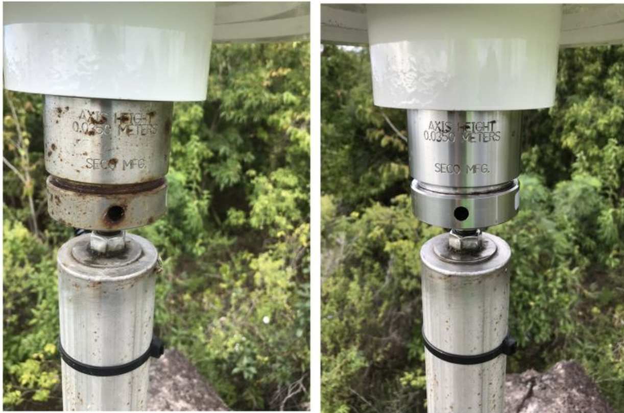
Fig 2. Corroded stainless steel leveller after 1 year of exposure to the elements at White Hook (left). After maintenance the leveller looks as good as new (right).
