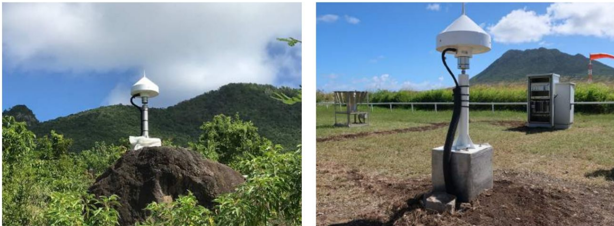
Fig. 1 GNSS installation by White Hook (left) and at the airport (right). The white part at the top is the antenna which receives the signals from satellites orbiting the Earth.
