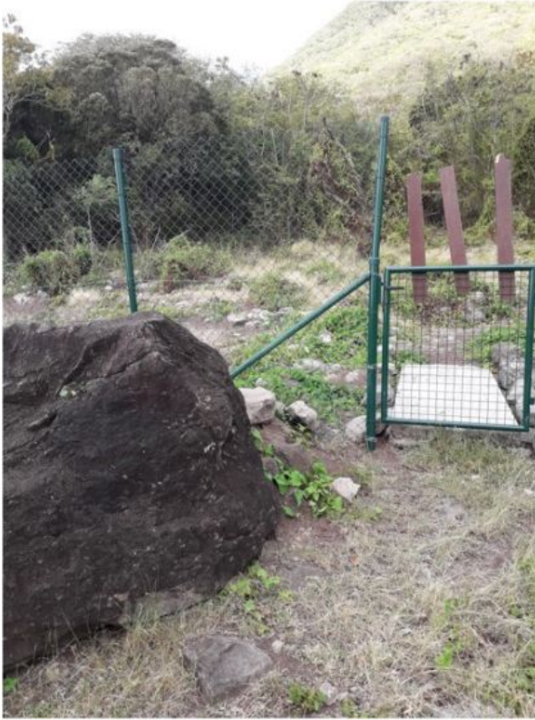
Fig. 3 Photos of the boulder on which the GNSS antenna, similar to the one at Wite Hook, would be placed (left) and the concrete slab which would house the vault for the GNSS receiver and seismometer (right).
