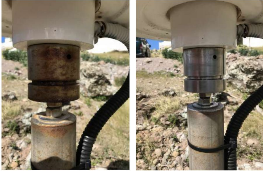
Fig 2. Corroded stainless steel leveller after 1 year of exposure to the elements at St. Johns (left). After maintenance the leveller looks almost new (right).
