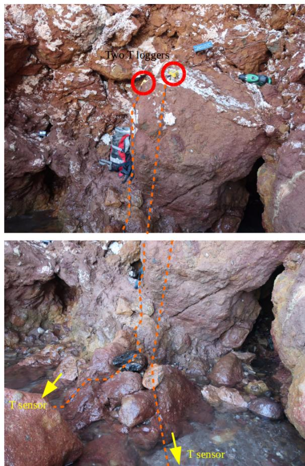
**Figure 14.** The hot spring opposite Green Island showing the attachment of two tinytag plus 2 data loggers to the cliff face and the cable path towards the submerged spring.
