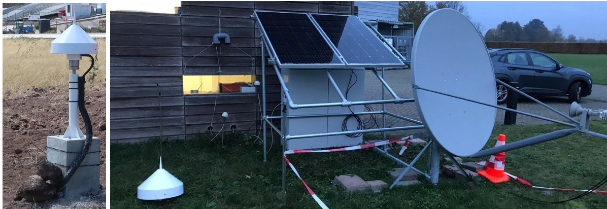
Fig.5: GNSS antenna mounted on a concrete monument (left). Concrete box for the seismometer not displayed. Test set-up at KNMI (right) showing VSAT dish, solar panels with cabinet underneath (5).
