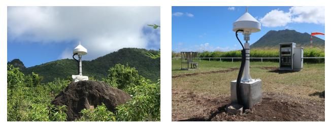
Fig. 1 GNSS installation by White Hook (left) and at the airport (right). The white part at the top is the antenna which receives the signals from satellites orbiting the Earth.
