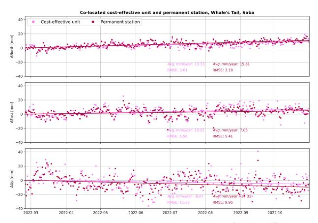
Fig. 5 Daily positioning results in North, East and Up direction of the cost-effective unit and the permanent GNSS at the Whale's Tail over a time span of 8 months. The movements to the North and East are caused by plate tectonics and are visible in data from both instruments. The error (RMSE) in the vertical (up) direction is also comparable.
