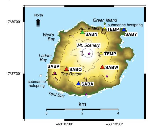
Fig. 1: Map showing the locations of current measurement sites on Saba with blue (GNSS/seismic stations) and red (seismic stations) triangles. The seismic and GNSS off-grid station is shown with a green triangle and the GNSS off-grid site with an orange triangle. Purple stars show the locations of the cost-effective units.
