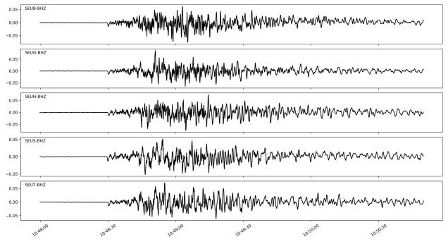
*Fig. 4:* Recordings of the vertical ground displacement (in millimeter) caused by the *M5.1* earthquake at 17-06-2022 10:48:12 UTC. This earthquake took place at a depth of about 40 km, about 100 km N of St. Eustatius.
