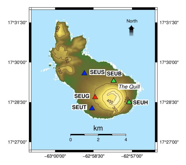
Fig. 1: Map showing the locations of current measurement sites on St. Eustatius with blue (GNSS/seismic stations) and red (seismic stations) triangles. GNSS/seismic stations that are self-sufficient are shown as green triangles.
