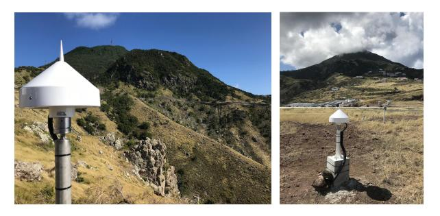
Fig. 1 GNSS installation by St. Johns (left) and at the airport (right). The white part at the top is the antenna which receives the signals from satellites orbiting the Earth.
