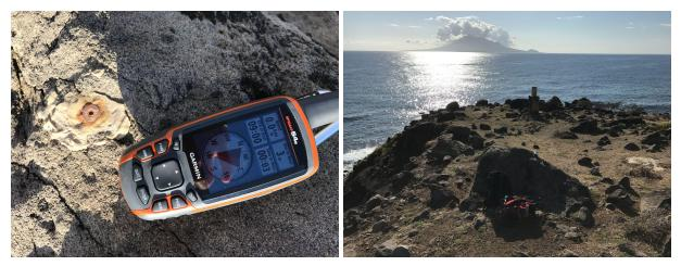
*Fig. 6: The campaign gravity site Hells Gate. The marker that is measured is the tiny pin to the left of the handheld GPS.*
