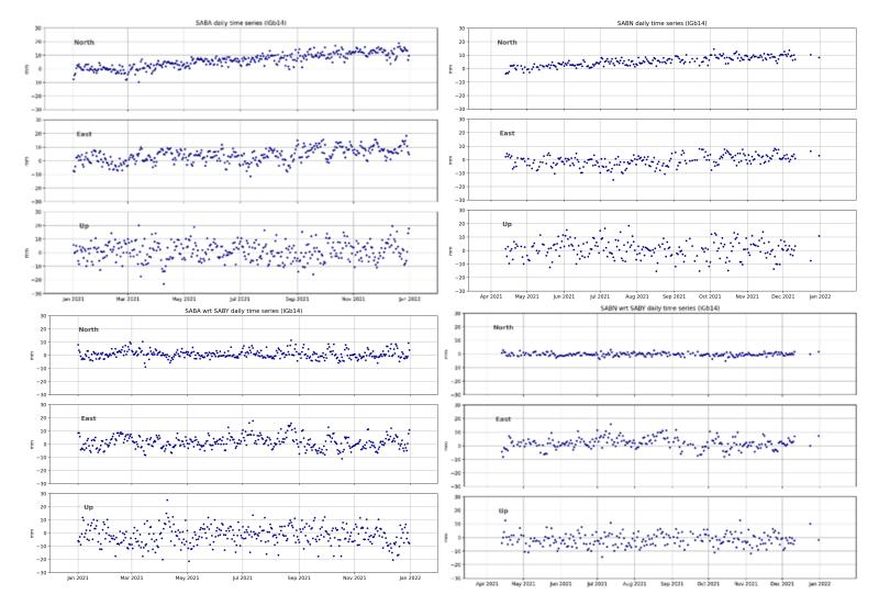
*Fig. 6:* GNSS data from stations SABA (upper left) and SABN (upper right) from 2021. When the plate movement signal is removed, the data shows very little deviation from a horizontal line (bottom graphs SABA and SABY).
