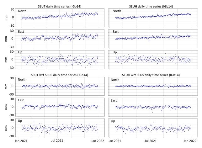
*Fig. 6:* GNSS data from stations SEUT (upper left) and SEUH (upper right) from 2021. When the plate movement signal is removed, the data shows very little deviation from a horizontal line (bottom graphs SEUT and SEUH).
