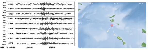
Fig. 5: Seismic recordings (left) from the seismometers at St. Eustatius of an automatically detected earthquake in between St. Eustatius and St. Maarten (right). The earthquake took place on 22-11-2021, 08:58:20 UTC, at a depth of 76 km and has a magnitude of 2.7.
