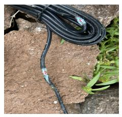
*Fig. 8: Chemical weathering of temperature sensor*
