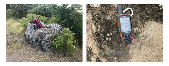
*Fig.9: The campaign gravity site Hells Gate. The marker that is measured is the tiny pin to the left of the handheld GPS.*
