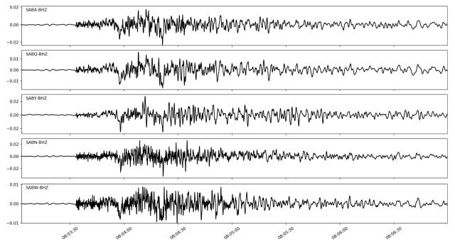
*Fig. 5:* Recordings of the vertical ground displacement (in millimeter) caused by the *M5.5* earthquake at 15-02-2022 08:03 UTC. This earthquake took place at a depth of about 50 km, about 240 km ESE of Saba.
