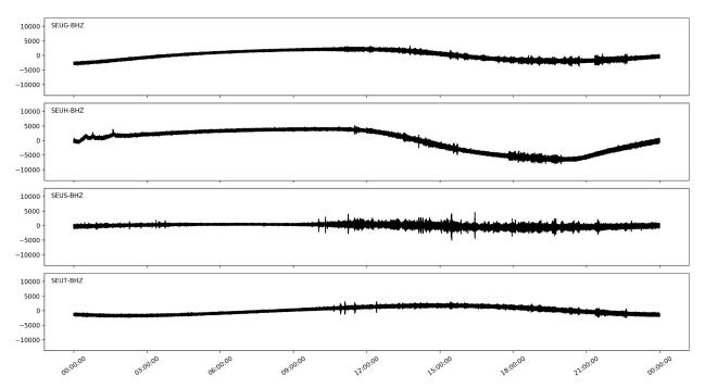
Fig. 4: Vertical ground motion recorded by the seismic stations at St. Eustatius on 01-09-2021. Notice the increase of human induced seismic noise during the day at SEUS due to its vicinity to traffic and offices. A daily variation, which is most likely due to temperature variation, is visible in SEUG and SEUH, and less pronounced in SEUT. Both the human induced noise and temperature variation do not limit the functioning of the seismometer and the detection of earthquakes.
