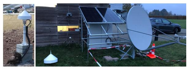
*Fig.5:* GNSS antenna mounted on a concrete monument (left). Concrete box for the seismometer not displayed. Test set-up at KNMI (right) showing VSAT dish, solar panels with cabinet underneath (5).
