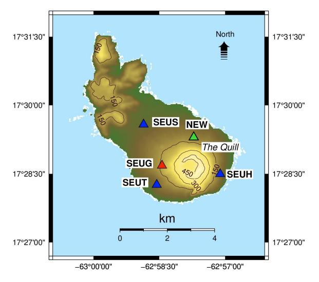
Fig. 1: Map showing the locations of current measurement sites on St. Eustatius with blue (GNSS/seismic stations) and red (seismic stations) triangles. Station SEUH was built in January 2021. In green the location of the proposed GNSS/seismic station at Bengalen (planned installation May 2022).
