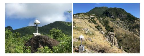
**Figure 12.** First continuous GNSS stations on St. Eustatius (**left**) with The Quill in the background and on Saba (**right**) in front of Mt. Scenery.
