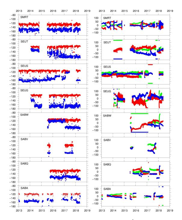
**Figure 7.** (a) Temporal variations of PSD (vertical component, dB rel. to  $m/s^2$ ) for 0.01 Hz (blue) and 1.0 Hz (red); (b) seismometer mass position for each triaxial, oblique component: U (green), V (red) and W (blue) [26]. Data gaps are visible as interruptions of different time lengths in both PSD and mass position graphs.
