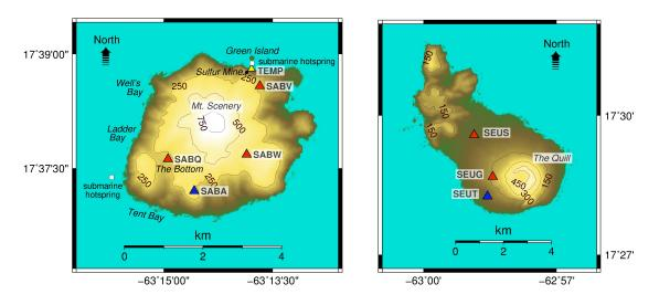
**Figure 2.** Geophysical monitoring network of the Royal Netherlands Meteorological Institute (KNMI) at Saba (**left**) and St. Eustatius (**right**): permanent sites with colocated seismometer and GNSS sensor (blue triangle), seismometer sites (red triangles), submarine hotsprings (white squares), and a temporary site with two temperature sensors (yellow triangle). SRTM Digital Elevation Model in the background with elevation contours in meters.
