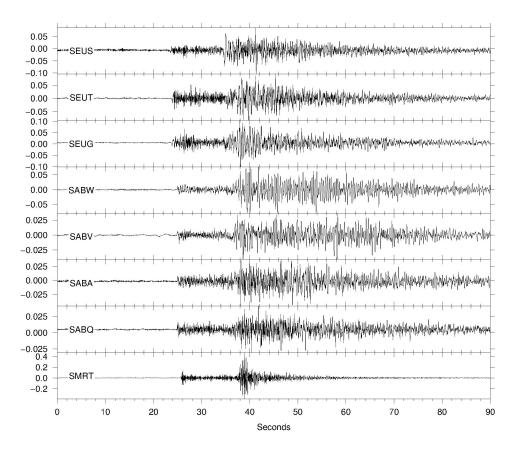
**Figure 5.** Example recordings of the vertical ground velocity (mm/s) by all eight NA stations of the magnitude 4.3 earthquake on 14 March 2017 at 18:35 UTC at a depth of 87 km just east of St. Eustatius. Stations are ordered by epicentral distance.
